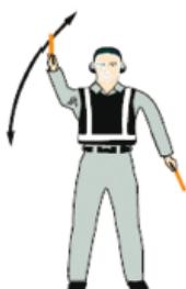
**14a. Turns while backing (for tail to starboard)**
