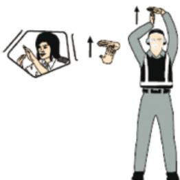
24. **Connect ground power (technical/servicing communication signal)**
