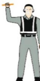
23. **Do not touch controls (technical/servicing communication signal)**
