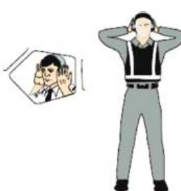
27. Establish communication via interphone (technical/ servicing communication signal)
