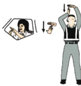
25. Disconnect ground power (technical/servicing communication signal)
